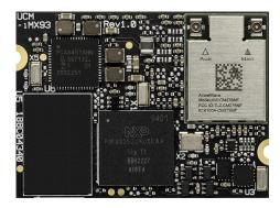
UCM-iMX93 is the very latest generation System on Module from NXP, delivered in an ultra-miniature form factor with energy flex architecture and state-of-the-art security to support energy-efficient edge computing.
